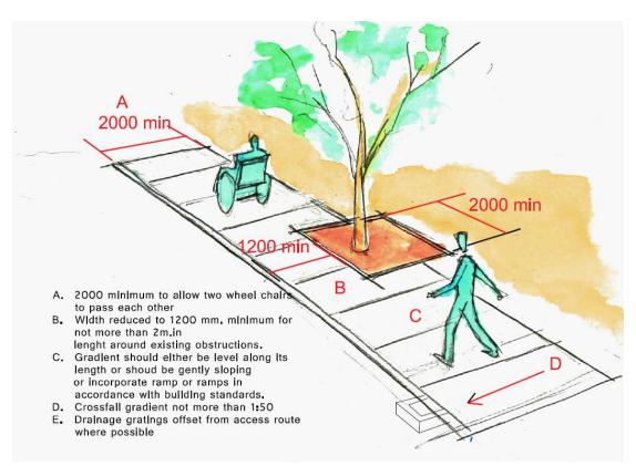
Figure 5. Urban environment pavement layout
