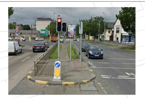
THE STAGGERED CROSSING IS GOING TO BE UPGRADED AS PER THE DESIGN PROJECT. ACCESSIBILITY MEASURES FOR CONTROLLED CROSSINGS SHOULD BE PROVIDED AND A PATH OF MINIMUM 1500MM. IF OBSTACLES CAN NOT BE REMOVED. 2000MM WIDTH RECOMMENDED.
