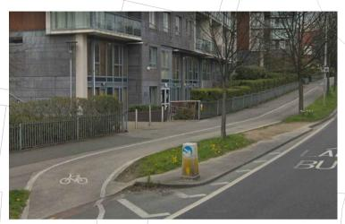
THE GRADIENT SHOULD BE CHECKED TO BE LESS THAN 1:20 (5%). WHERE A GENTLY SLOPED ACCES ROUTE IS PROVIDED: (GRADIENT STEEPER THAN 1:50 AND LESS THAN 1:20) PASSING PLACES FOR WHEELCHAIR USERS SHOULD BE PROVIDED (2000MMx1800MM). IF THE ACCESS ROUTE IS MORE THAN 25M. SOME RESTING PLACES OR BENCHES SHOULD BE ALSO RECOMMENDEDT SHOULD BE REPAIRED WITH A PROPER PAINT MARKS.
