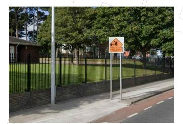
THE POSITION OF THE SIGNAGE SHOULD BE REVIEWED TO FACILITATE THE MANEUVERING OF PEOPLE WITH DISABILITIES MINIMUM WIDTH OF FOOTPATH 1200 MM. IN A DISTANCE OF 2000MM,
