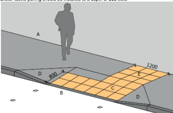
Figure 11. Uncontrolled Crossing at Side Road
