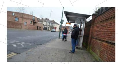
BUS STOP. LACK OF TEXTURED SURFACE AT THE EDGE BOUNDARY AND ABSENCE OF A KASSEL KERB FOR ADAPTING MODERN BUSES AND THEIR KNEELING SUSPENSION.
