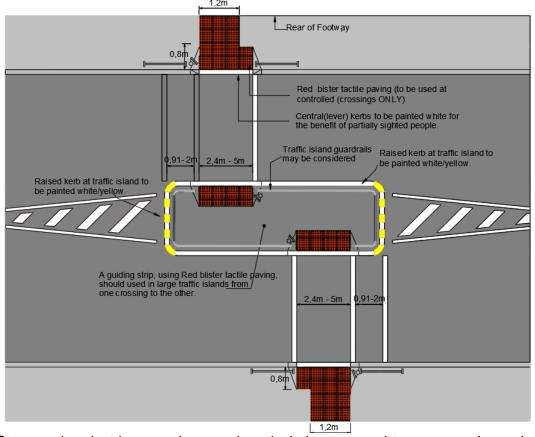
Staggered pedestrian crossings, and particularly staggered toucan crossings where they exist, shall be designed out as per the Design Manual for Urban Roads and Streets [DMURS]. The space provided within the islands of staggered crossings is generally constrained and difficult for vulnerable pedestrians to navigate. Single stage crossings should be provided to improve dwell space, crossing legibility and to reduce crossing distances.
