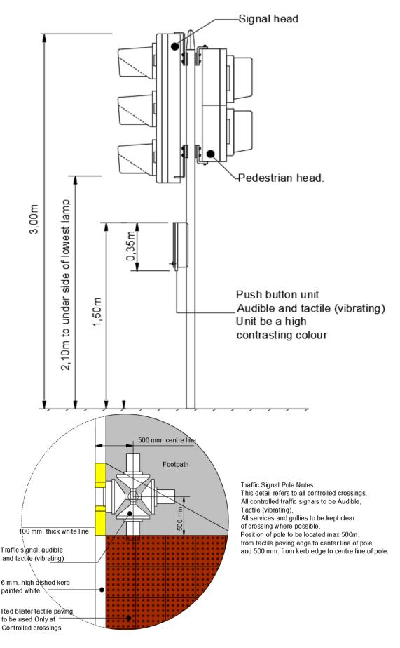
Figure 23. Plan and Elevation of traffic Signal
