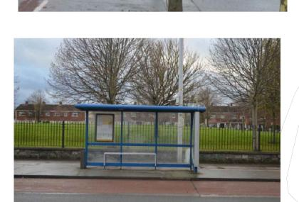
BUS STOP. A KASSEL KERB SHOULD BE INCORPORATED AND TEXTURED SURFACE TO WARN PEOPLE WITH VISUAL IMPAIRMENTS. THE OPTIMUM KERB HEIGHT AT A BUS STOP TO CATER FOR THESE PERSONS SHOULD BE AROUND 180MM. AN ISLAND BUS OPTION SHOULD BE CONSIDERED FOR AVOID THE PEDESTRIAN/CYCLIST CONFLICT, WITH AN ON-DEMAND SIGNALISED PEDESTRIAN CROSSING (TACTILE PAVING; PUSH BUTTON, LED WARNING STUDS) AND A SECONDARY UNCONTROLLED CROSSING ON THE DOWNSTREAM OF THE ISLAND.
