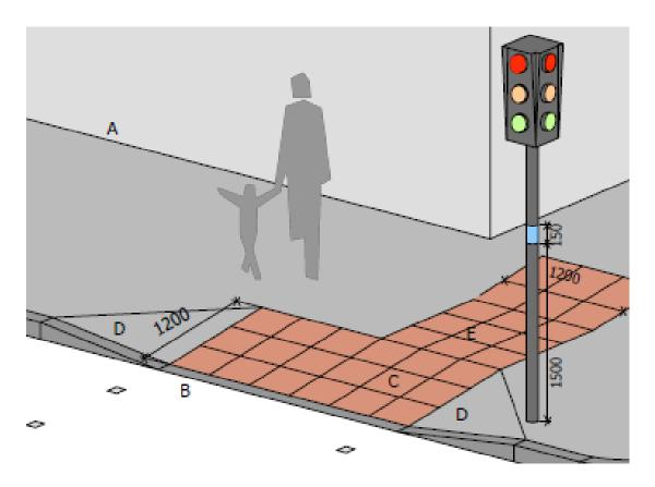
Figure 16. Controlled Crossing. In Direct Line of Travel
