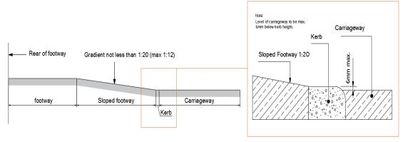
Figure 8. Dished Kerb Section Detail
