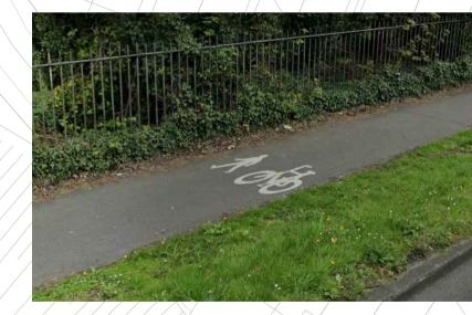
CONFLICT IN THE SHARE ROUTE (PEDESTRIAN/CYCLIST). NO SEGREGATION AND ENOUGH WIDTH BETWEEN THEM IN THIS PART OF THE ROUTE. WIDTH OF 1500 MM WHEN OBSTACLES CAN NOT BE REMOVED. A CYCLING FACILITY SEGREGATION (HORIZONTAL AND VERTICAL) IS RECOMMENDED.
