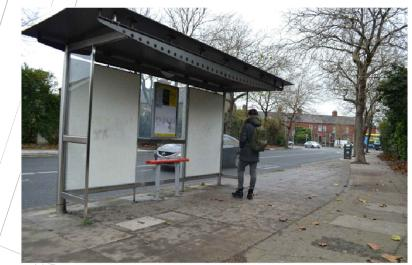
SHELTER IS PLACED IN SUCH POSITION THAT THERE IS NO GOOD VISIBILITY FOR BUSES AND PEOPLE WAITING. CORRECT LOCATION OF THE SHELTER SHOUD BE REVISED. KASSEL KERB TO BE INCORPORATED. FOR THE DESIGN PROPOSAL A ISLAND BUS OPTION WOULD BE THE PREFERRED. WITH CONTROLLED/ OR UNCONTROLLED CROSSING BETWEEN FOOTPATH AND CYCLE TRACK
