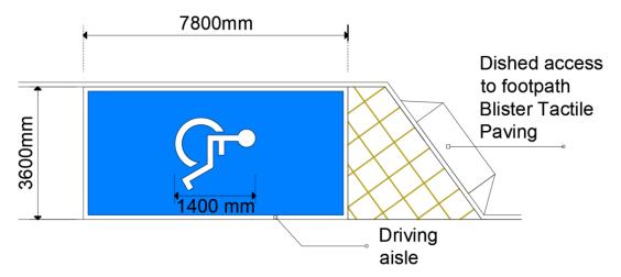
Figure 3. Example of Parallel parking
