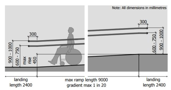
Figure 25. Examples of external ramp
