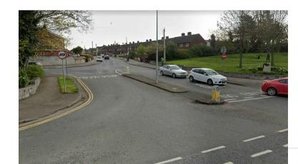
UNCONTROLLED CROSSING. A DISHED KERB AND "BUFF" OR GREY TACTILE PAVING SHOULD BE CONSIDERED. DEPTH OF 1.2 M, GRADIENT 1:12 MAX. LEVEL DIFFERENCE OF DISHED KERB: 6MM. IN THE DESIGN PROJECT A CONTROLLED CROSSING IS PROPOSED. ACCESSIBILITY MEASURES FOR THIS TYPE OF CROSSING SHOULD BE IMPLEMENTED.
