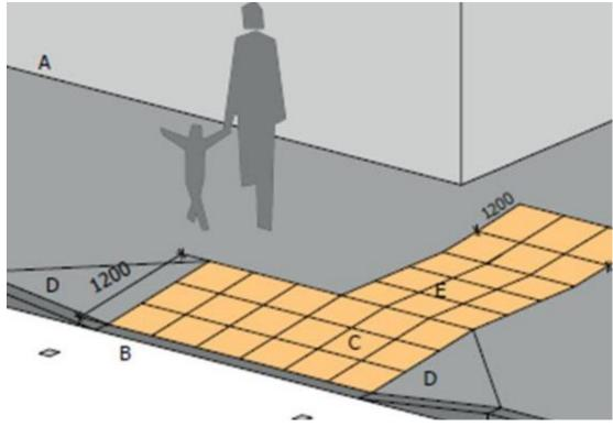
Figure 9. Uncontrolled Crossing. In line
