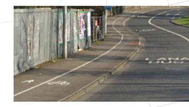
CHECK CORRECT WITDH OF FOOTPATH IN THE SHARED ROUTE, MINIMUM 1500 MM. WIDTH WHEN OBSTACLES CAN NOT BE REMOVES. A CYCLING FACILITY SEGREGATION (HORIZONTAL AND VERTICAL) IS RECOMMENDED.
