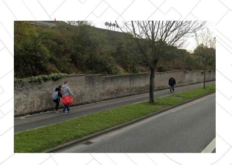
CONFLICT IN THE SHARE ROUTE (PEDESTRIAN/CYCLIST). NO SEGREGATION AND ENOUGH WIDTH BETWEEN THEM IN THIS PART OF THE ROUTE. WIDTH OF 1500 MM WHEN OBSTACLES CAN NOT BÉ REMOVED. A CYCLING FACILITY SEGREGATION (HORIZONTAL AND VERTICAL) IS RECOMMENDED.
