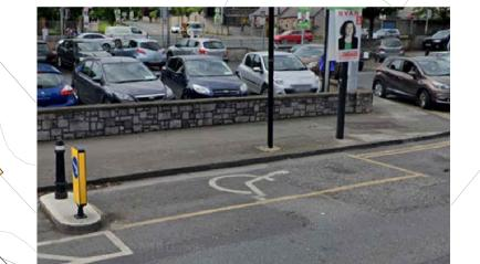
ON STREET CAR PARKING SPACE, NO DISHED KERB AND DIMENSIONS 3,6 x7m. MEASURES FOR ACCESSIBILITY PARKING BAYS IN PARALLEL SHOULD BE IMPLEMENTED.
