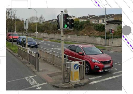
STAGGERED CROSSING POINT SHOULD BE REVIEWED. A SOLUTION OF A FULL-WIDTH CROSSING IN ONE STAGE SHOULD BE CONSIDERED TO AVOID PEOPLE WITH DISABILITIES GET STUCK IN THE NARROW AREA OF CENTRAL REFUGE.
